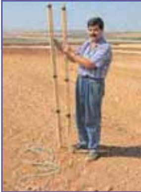
The tube level is used to locate the contour precisely before ridge construction. Low in cost and easy to use by farmers.
