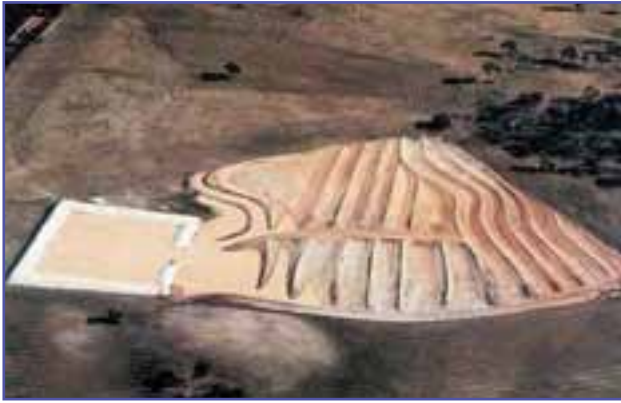
Inter-row system concentrating runoff water in a reservoir in Australia. Photo from booklet on water harvesting by the State Department of Western Australia.
