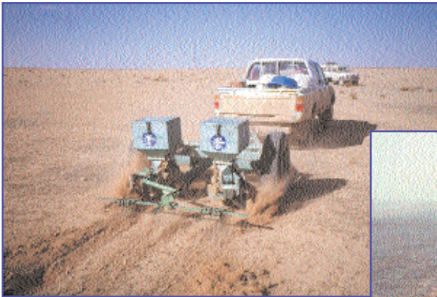
Left: The Kimseed pitting machine adapted by ICARDA for use in West Asian environments
