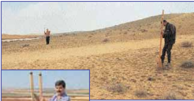
The tube level is used to locate the contour precisely before ridge construction. Low in cost and easy to use by farmers.
