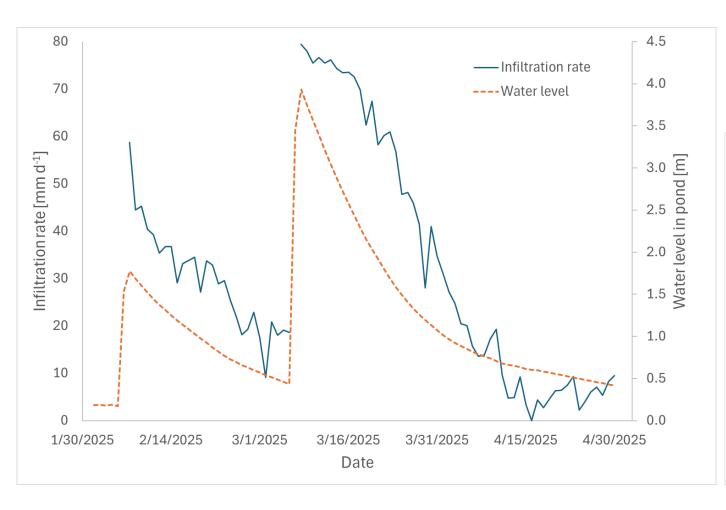
Total infiltration in Al-Muwaqqar pond is 2,777 mm in 89 days
