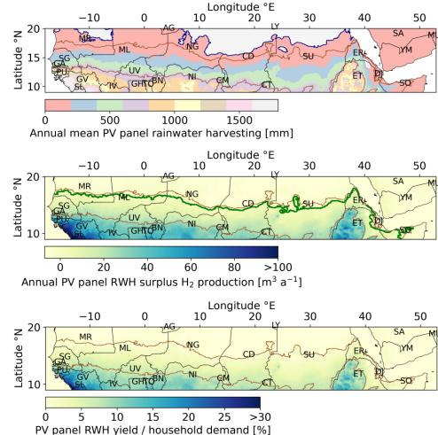
Where precipitation exceeds 200 mm a<sup>-1</sup> combined solar energy and rainwater harvesting has potential to increase available water resources in the Sahel Region. High water gains are obtained when energy is harvested for H<sub>2</sub> production
