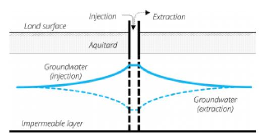
Gravitational recharge through shallow or deep structures such as dry wells, shafts, boreholes or pits.
