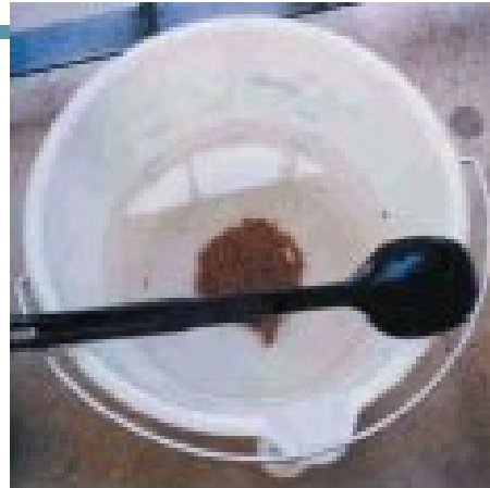
Floc formation after complete stirring
