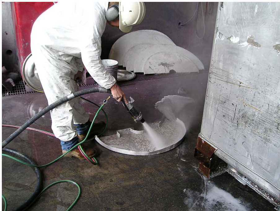
Fig. 2. Trimac has eliminated 100% (24 tonnes/year) of methylene chloride use by changing to a baking soda and compressed air blasting process.
